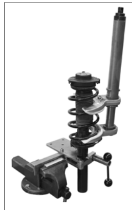
Fig. 8: Clamping a suspension-/damper strut into holding fixture.
